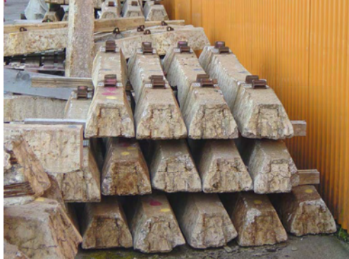
Figure 6.2 Picture showing how the sleepers have been stored during the period November 2000 – June 2003, Thun & Elfgrén (2003).
