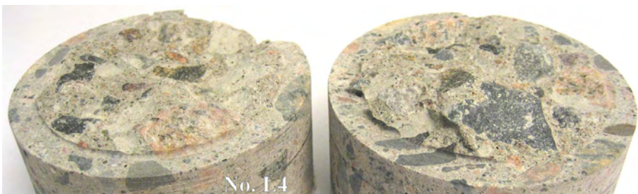
Figure A.41 Photograph showing the failure surface for test No. L4 after fatigue test. A part of the notch has loosened.
