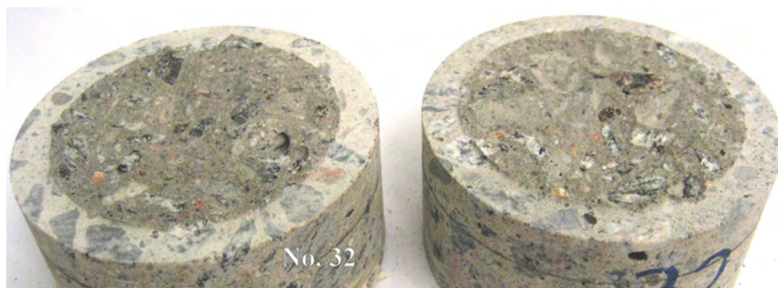
Figure A.30 Photograph showing the failure surface for test No. 32 after fatigue test.
