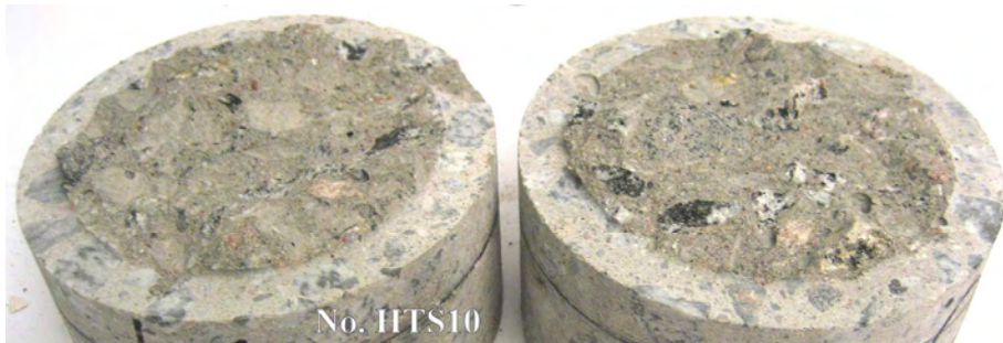
Figure A.39 Photograph showing the failure surface for test No. HTS10 after tensile test.
