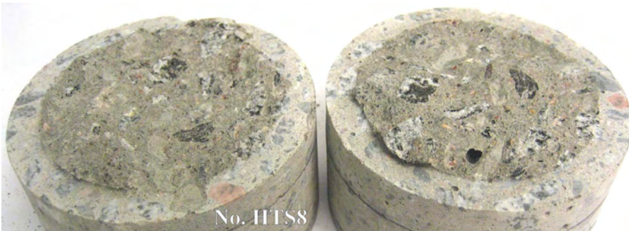
Figure A.37 Photograph showing the failure surface for test No. HTS8 after tensile test.
