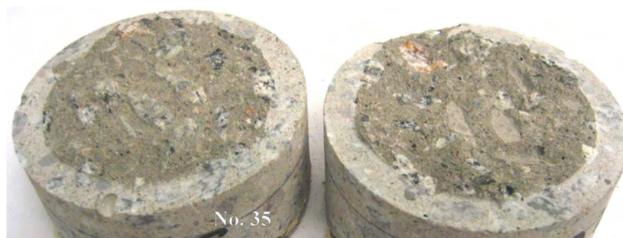
Figure A.33 Photograph showing the failure surface for test No. 35 after fatigue test.
