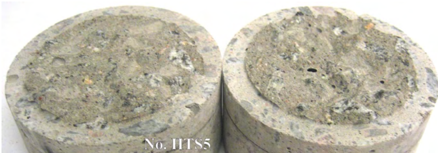
Figure A.35 Photograph showing the failure surface for test No. HTS5 after tensile test.
