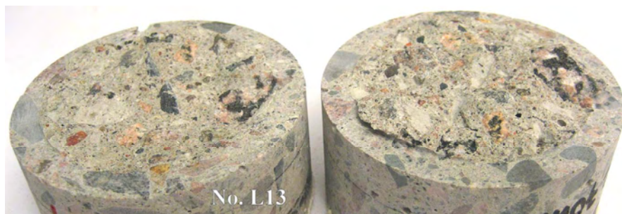
Figure A.49 Photograph showing the failure surface for test No. L13 after fatigue test.
