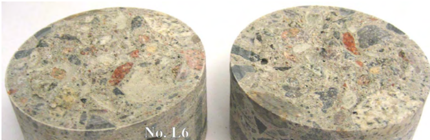
Figure A.43 Photograph showing the failure surface for test No. L6 after fatigue test.
