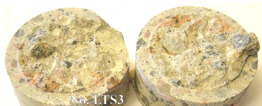
Figure A.55 Photograph showing the failure surface for test No. LTS3 after tensile test. Large stone in the notch. 1/4 of the notch loosened.
