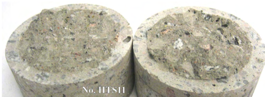
Figure A.40 Photograph showing the failure surface for test No. HTS11 after tensile test.
