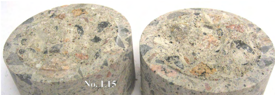
Figure A.51 Photograph showing the failure surface for test No. L15 after fatigue test.
